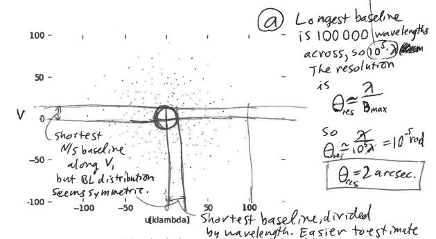
If this observation was at 230 GHz at zenith, what is the approximate resolution of the observation? What is the smallest separation (in meters) between two antennae in the N/S direction?
